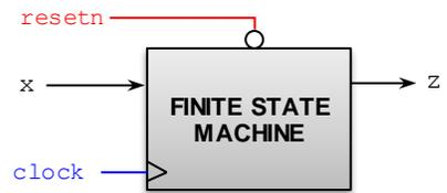
State Assignment: S0: Q=00, S1: Q=01, S2: Q=10, S3: Q=11
